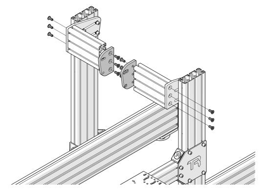
Note: Use screws and t-nuts provided with wheelbase.
